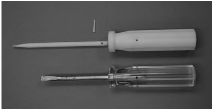
3D printed (top) and machined (bottom) versions of a screwdriver
